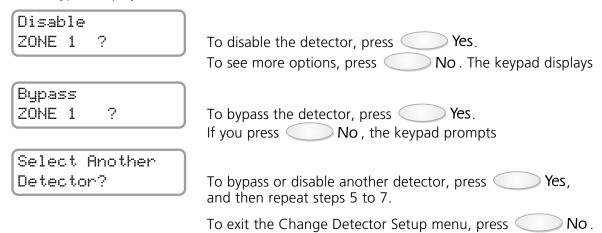
Step 8. If you have bypassed or disabled any of the detectors, the keypad displays:
