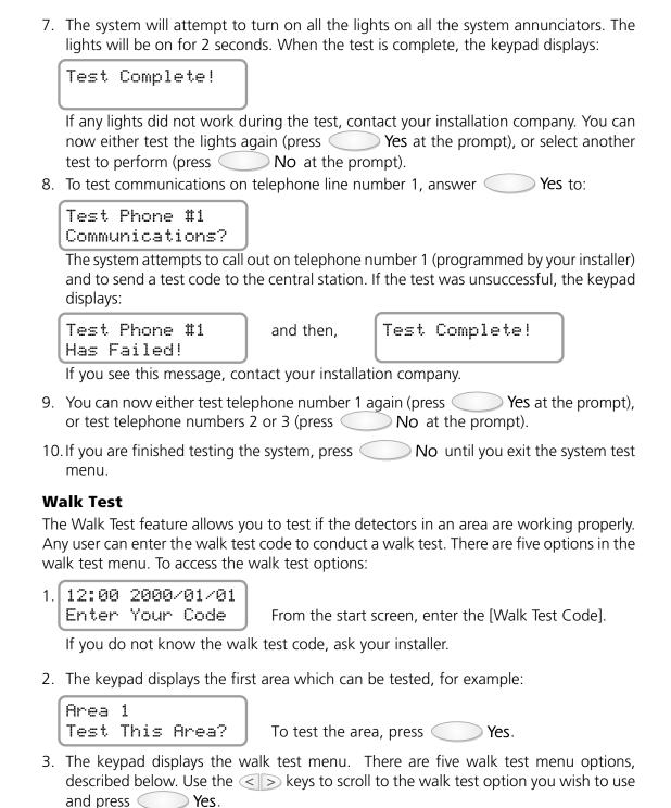
For motion detectors, create movement in the detected area. For door and window contacts, open and close protected doors and windows. Any open zone will cause the bell or siren to sound for two seconds, confirming that the detectors are working properly.
